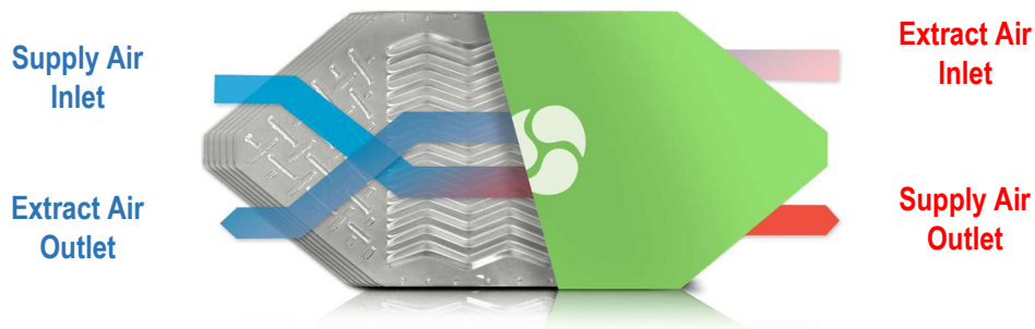
Air flow diagram of PCF counterflow heat exchanger
